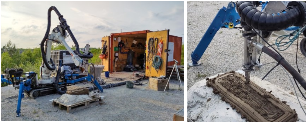
Fig. 2. A: Construction Robotics Lab. B: Clay extruder connected via hose to pump.
